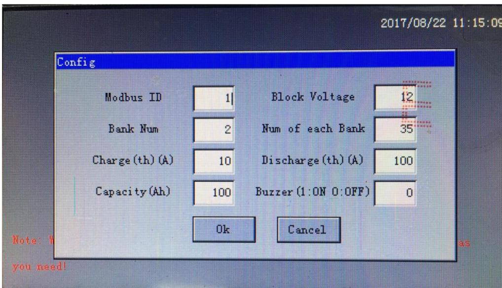
Modbus ID: If connected with multiple sets of control module, the modbus ID of each control module cannot be repeated, it requires to modify the Modbus ID from here.
