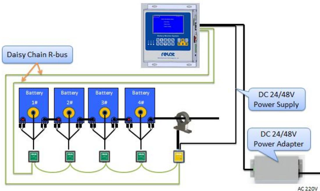
Till now, all the installations is complete. Check all the connections of battery sensor, I-Sensor and Control Module, to make sure all are correct, especially the positive and negative terminal of batteries and power, before power on them.
