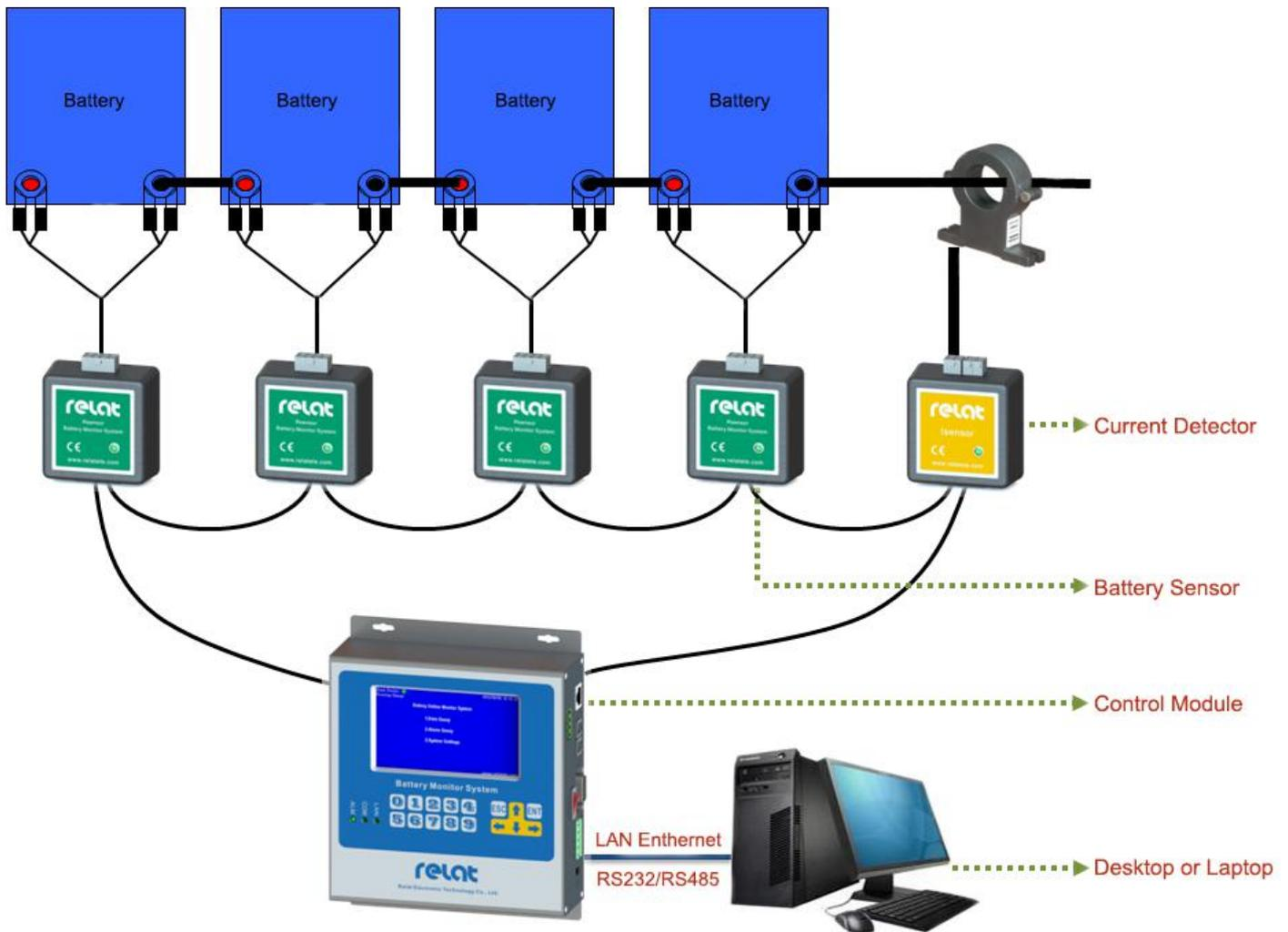
The Relat Battery Monitoring System(BMS) is composed of the control module, current detector and the battery sensor. Please check the BMS Component List below,
