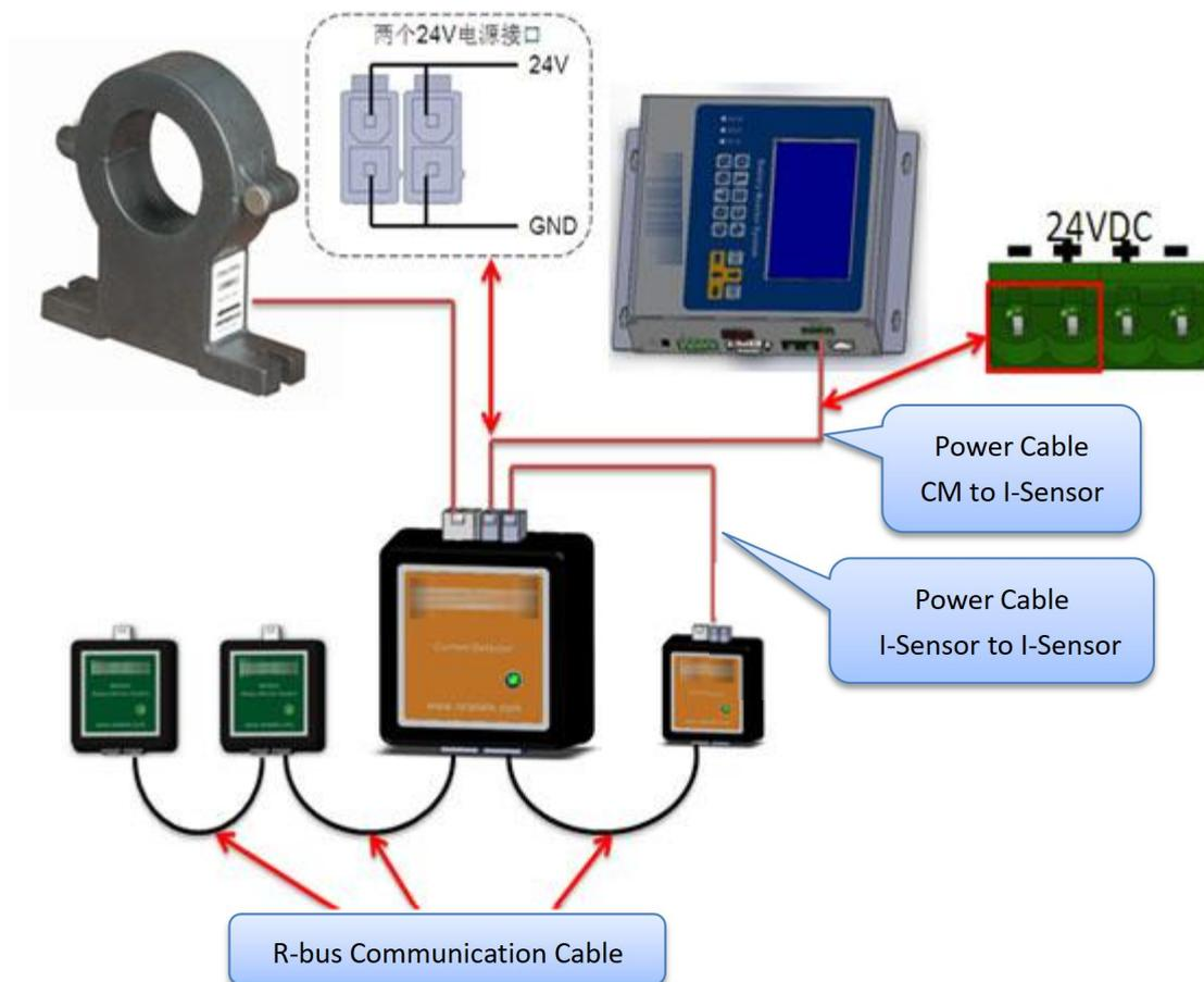
Make sure the current transformer is in correct direction.
