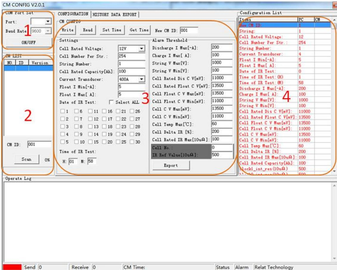
**Step 1:** Select COM Port and press ON/OFF, the status will show green color instead of red, when the connection has been established.
